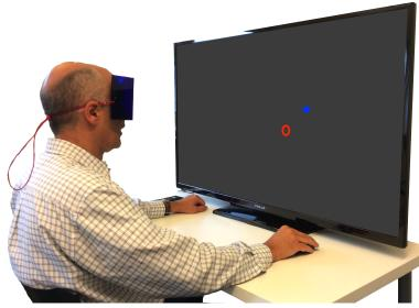
KMScreen T55 is made up of a 55 inch TV screen and a minicomputer with pre-installed software. It is possible to connect an extra monitor to your computer, so that the examiner can control the program and observe and follow the test results following every click from the patient.
